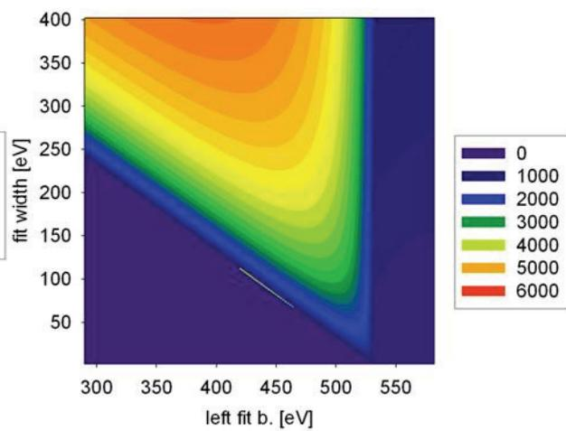
Fig. 2 Optimization of the SNR calculated with the MLS method plotted as function of the size and position of the fitting window.
