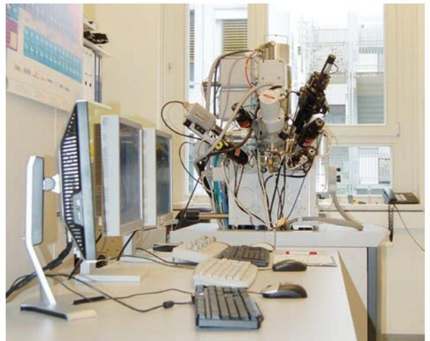
Focused ion beam microscope FEI Nanolab NOVA 200.
