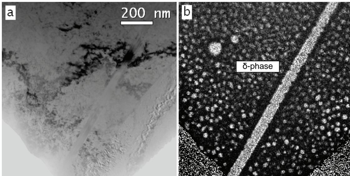
Fig. 1a) TEM bright field image of Allvac 718 Plus<sup>TM</sup>, b) EFTEM Ni-M<sub>2,3</sub> jump ratio image.
