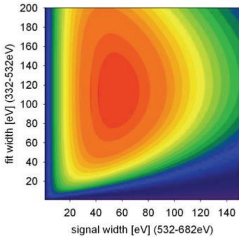
Fig. 1 Optimization of the conventional calculated SNR plotted as function of the size of the fitting window and the signal window.
