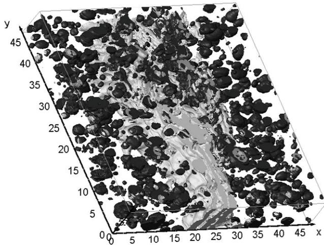
Fig.2 3D-representation of EPR (ethylene propylene rubber) modified iPP (isotactic polypropylene) after a tensile test, stopped at 25% yield and stained with  $\text{RuO}_4$  (160 slices, slice thickness: 100 nm); black: EPR particles; grey: cracks.
