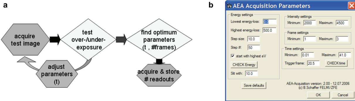
Fig.1. Simplified flow diagram (a) and user interface (b) of an EFTEM spectrum image acquisition process, which automatically adjusts for dynamic range differences in the EELS spectrum.
