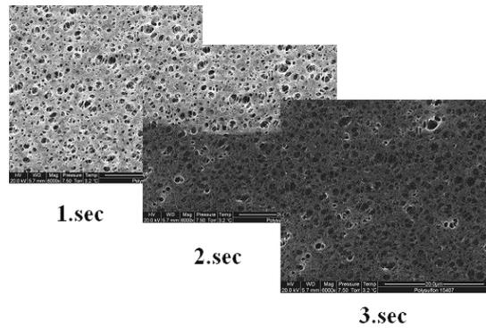
Fig.3 Wetting of a polyethersulfon membrane (nominal pore size: 450 nm) with water in dependence on time (width of the images: 45  $\mu\text{m}$ ). Some of the big pores remain partially filled / unfilled. The water was provided by condensation at a Peltier cooling stage.
