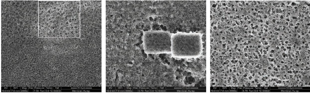
Fig. 1 Wetting and drying-up of a cellulose nitrate membrane (10 nm Au-coating). Left: Before recording the image, mainly the marked area had been irradiated. Contrary to the surrounding, many of the pores in this area are not filled / fully filled with water (image width: 100  $\mu\text{m}$ ). Centre and right: Drying-up is delayed in the irradiated areas (centre) compared to other areas (right). In the irradiated areas strong damage is visible (image width: 42  $\mu\text{m}$ ).
