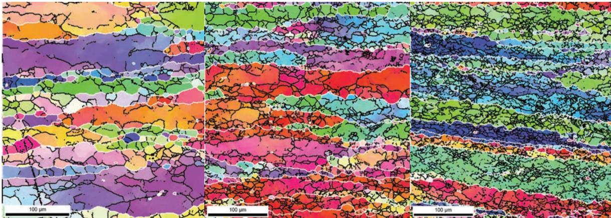
Fig. 1 Inverse pole figure maps (IPF) of the compressed specimens at  $T = 550^{\circ}\text{C}$  and  $\dot{\phi} = 1\text{s}^{-1}$  (left) respectively  $\dot{\phi} = 10\text{s}^{-1}$  (centre), as well as  $T = 500^{\circ}\text{C}$  and  $\dot{\phi} = 10\text{s}^{-1}$  (right); white lines mark the high angle boundaries ( $>15^{\circ}$ ) and black lines the subgrain boundaries (between  $2^{\circ}$  and  $15^{\circ}$ ).
