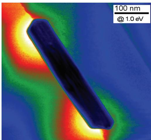
Distribution of surface plasmons around an Au nanorod, recorded with the monochromated FEI Tecnai F20.
