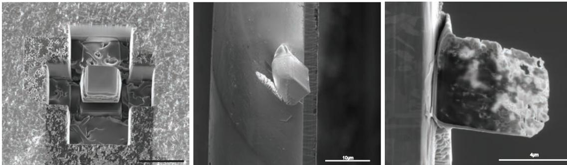
Fig. 2 a-c. SEM images of the plane view preparation in the focused ion beam instrument (FIB).
