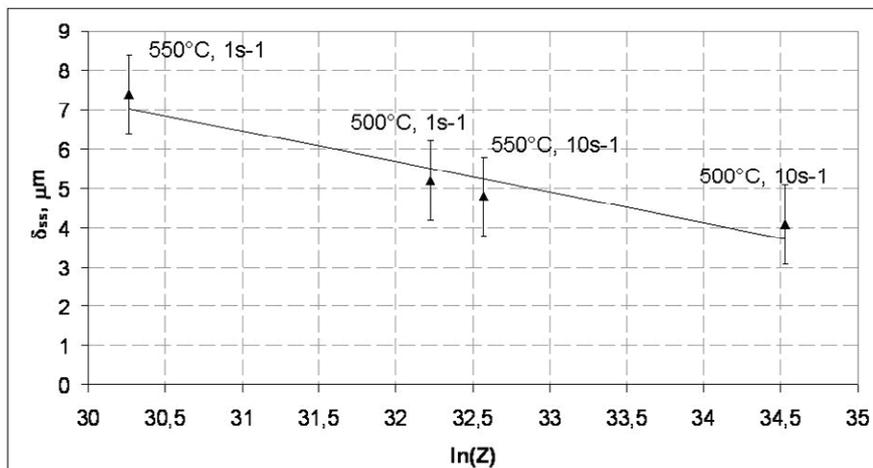
Fig. 2 Size of the subgrains (experimentally determined) in dependence on the Zener-Hollomon-parameter.
