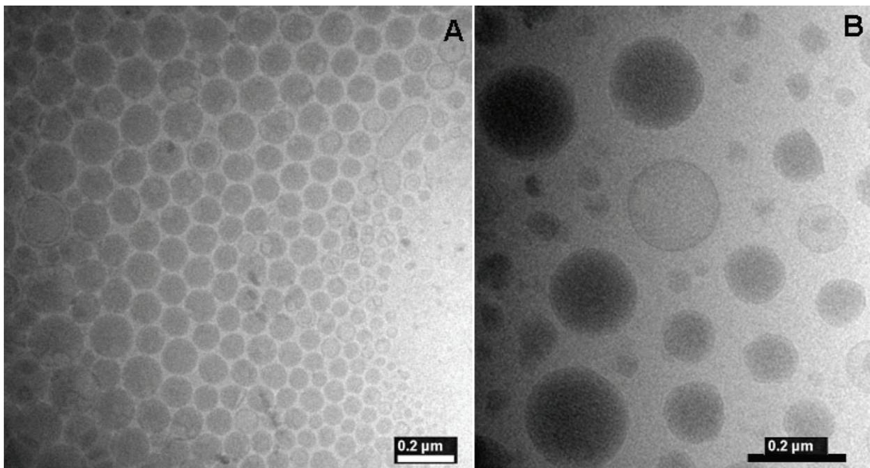
Fig. 2 (A) Cryo TEM of oil/water nanoemulsions (sample from Viktoria Klang, TU Wien) and (B) monolinolein (MLO) / water nanostructured dispersions.
