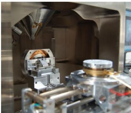
The specimen stage of the Zeiss Ultra 55.
