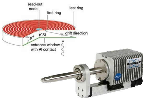
The silicon drift detector for the focused ion beam microscope (XFlash<sup>®</sup> Bruker AXS).
