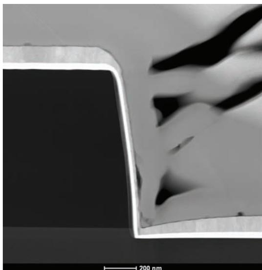
STEM-HAADF image of a cross-section of a semiconductor recorded with the FEI Tecnai F20.
