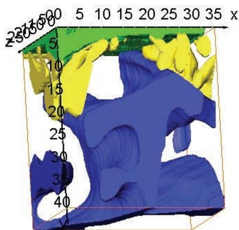
3D-elemental map of a casting alloy, presented as an RGB-image; green = silicon, blue = aluminium, yellow = iron; in  $\mu\text{m}$
