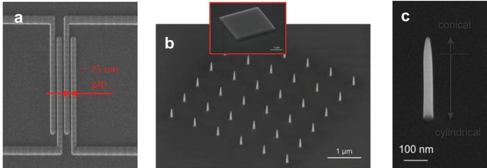
Fig. 1 Scanning electron microscopy images of electron beam induced deposition of defined Pt nanostructures (a), single elements (b) of larger deposits (inset), and intrinsic morphologies of a single Pt nano-rod (c).
