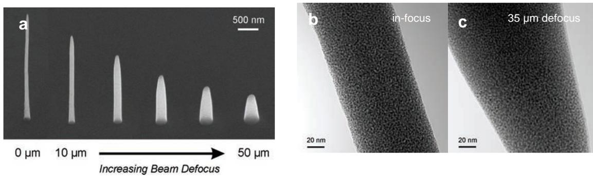
Fig. 2 Influence of beam defocus during deposition on the morphology of Pt single nano-rods (a, scanning electron microscopy images). Structural composition of Pt nano-rods for in-focus (b) and 35 μm defocus (c) conditions (transmission electron microscopy images).
