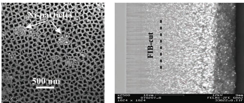
Fig. 2 Left: TEM-image of a FIB cut Ni-filled PS-sample showing precipitated Ni-particles within the pores of the PS-matrix. Right: Cross-sectional SEM-image of the entire porous layer of same sample. The level of the FIB-cut is marked.
