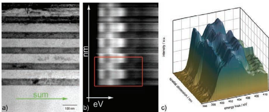
Fig. 3 EFTEM SI data at the N-K edge of GaN/AlN: a) Bright-field image showing the sample; b) EFTEM SI averaged along spatial x-direction - green arrow in a) - and plotted energy vs. spatial y-direction; c) 3D display of N-K ELNES across four layers - red area in b).
