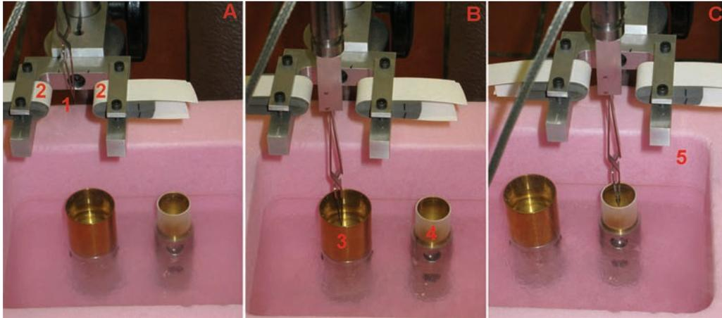
Fig. 1 Vitrification of the sample. A small aliquot of a fluid suspension is applied to the surface of a holey carbon film that is attached to the surface of a standard TEM specimen grid (A (1)). The droplet is blotted with filter paper (A (2)). After the grid is plunged into the ethane pot (B (3)), and then is transferred into liquid nitrogen pot (B (4)), the workstation (C (5)) is removed and the grid transferred to a pre-cooled cryo transfer holder for immediate viewing on the TEM.
