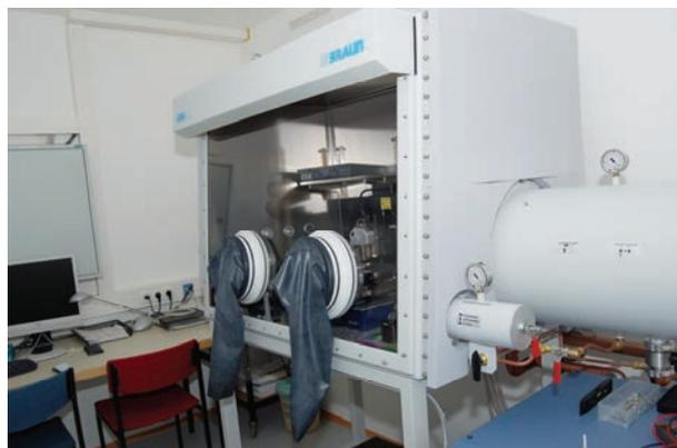
Atomic force microscope VEECO Dimension in the glove box.
