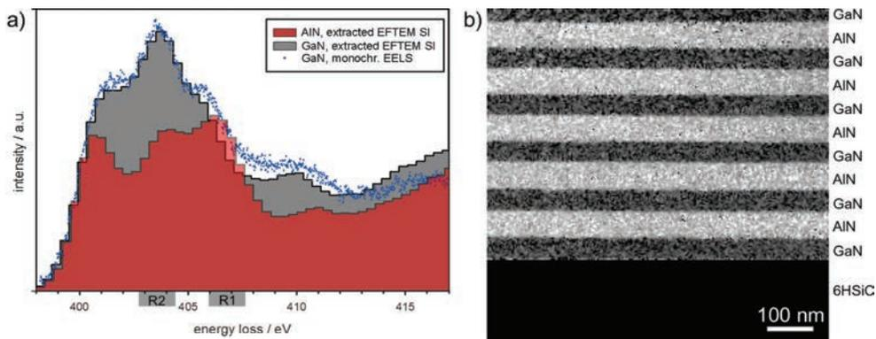
Fig. 2 a) ELNES of the N-K edge of GaN and AlN extracted from EFTEM SI. GaN data acquired in monochromated spectroscopy mode is added for comparison; b) N-K ELNES jump ratio image extracted from EFTEM SI. The energy ranges of the jump ratio image R1/R2 are indicated in a).
