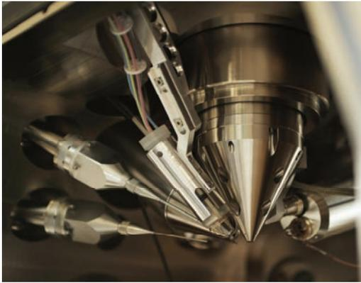
Specimen stage of the focused ion beam microscope FEI Nanolab NOVA 200.
