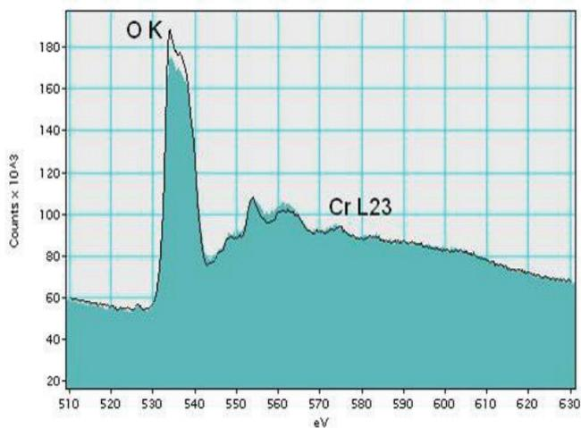
Fig. 3 EEL spectrum of ruby (filled area) with the appropriate MLS Fit (black line). Cr 0.4at%
