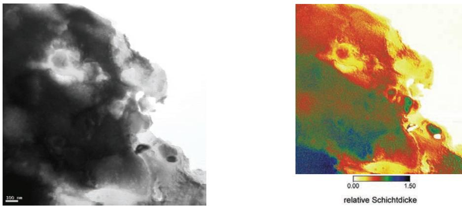
Fig. 3. TEM BF image of extraction replica with permanent polymer and EFTEM thickness map.
