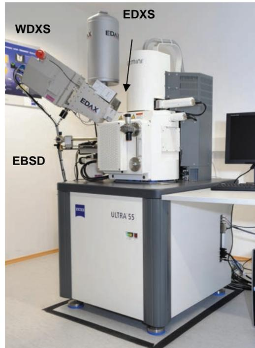
The column of the Zeiss Ultra 55, now equipped with an EDXS-, WDXS- and EBSD-spectrometer.
