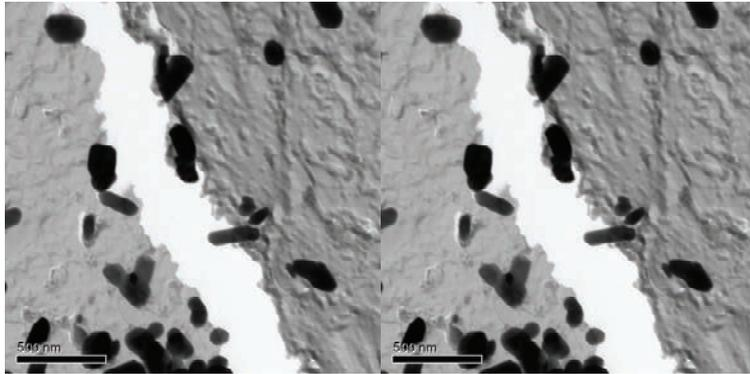
Fig. 1 TEM BF image of pre-etched precipitates covered with a carbon film.
