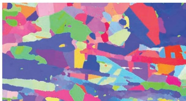
EBSD map of crystal grains in a duplex steel; colors indicate different crystal orientations; image length = 10  $\mu\text{m}$ .
