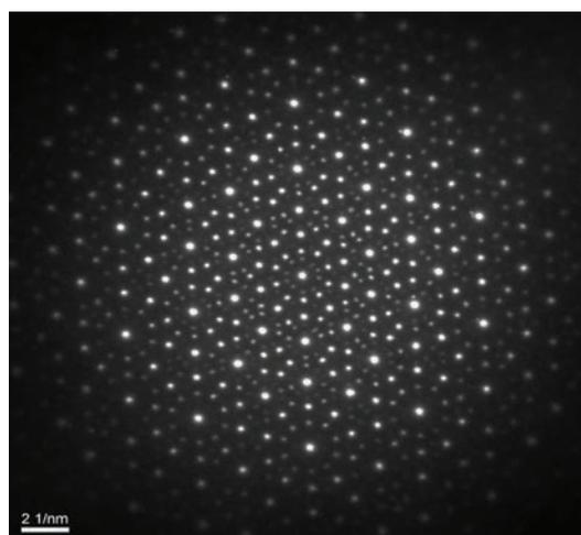
Electron diffraction pattern of a quasicrystalline phase in a melt-spun Al-Mn-Be alloy (sample courtesy, F. Zupanič, University of Maribor, Slovenia).
