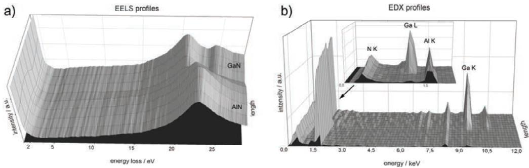
Fig. 1 Line scan across the interface of a GaN / AlN multilayer sample extracted from simultaneous EELS/EDX STEM SI: a) EELS low-loss spectra; b) EDX signal
