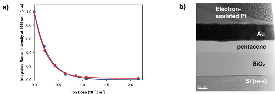
Fig. 1 a) Raman curves showing a similar irradiation behavior at room and cryo temperature of P3HT thin films towards increasing ion doses, b) TEM cross-section image of an organic thin film transistor.
