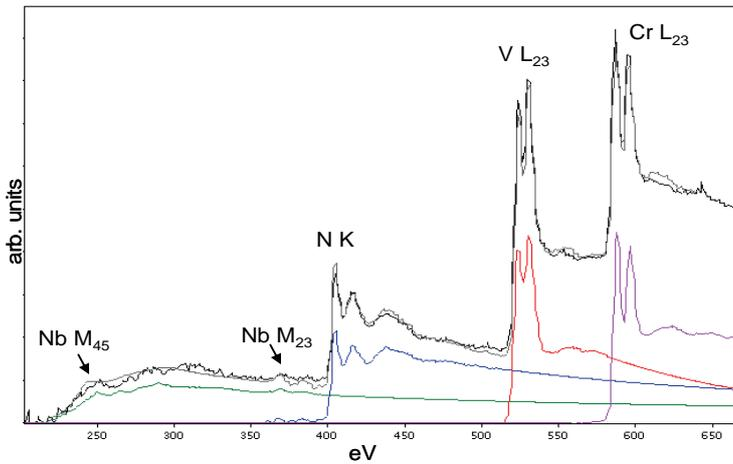
Fig. 2 MLS fit using Nb, N, V and Cr - references for a mod. Z-phase particle; the experimental spectrum is represented in black and the MLS fit in grey.
