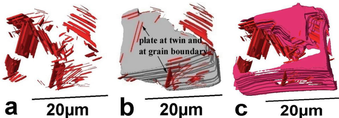
Fig. 2a) Reconstruction of the  $\delta$ -phase, b) twin-reconstruction with the  $\delta$ -phase and c) surrounding grain with the  $\delta$ -phase.
