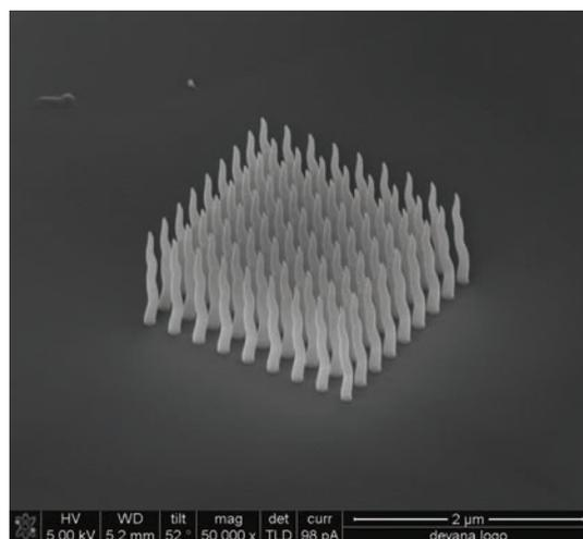
Pt nanowires prepared in a focused ion beam microscope (FIB) using the electron beam.
