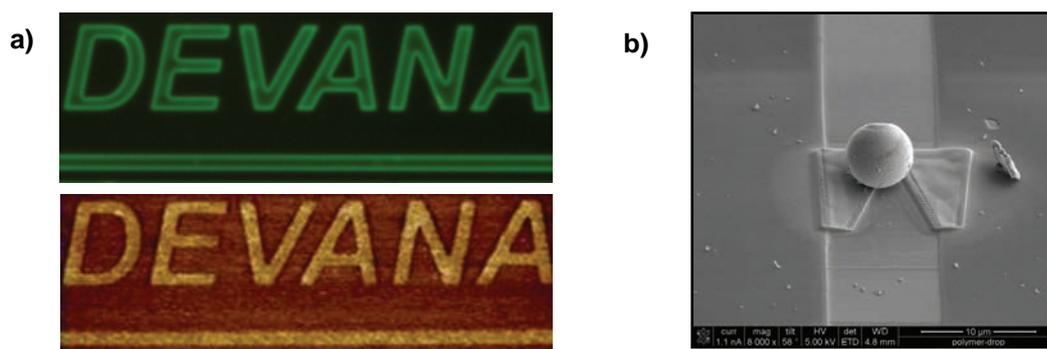
Fig. 2 a) The PL and KPFM image of an electron-beam-patterned logo on a PF thin film; the emission color was tuned from blue to green using EB irradiation, b) nano-LED structure, fabricated by in-situ FIB prototyping.
