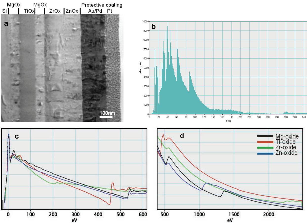
Fig.2. a) Oxide multilayer stack and b) example of an unscaled, raw EFTEM SI spectrum, reflecting different exposure times and number of image summations at different energies; c) and d) logarithmic representations of corrected spectral data spanning from the zero-loss peak to Zr-L<sub>2,3</sub> at 2.2 keV.
