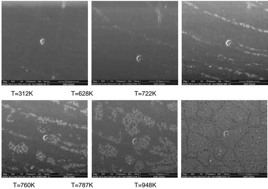
Fig. 1 Observation of scale formation during heating in the ESEM
