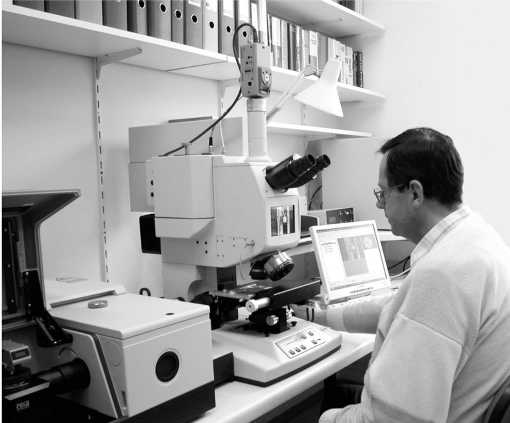
Dr. Peter Wilhelm working with the new FT-IR microscope Bruker Equinox 55 spectrometer with Hyperion 3000 microscope
